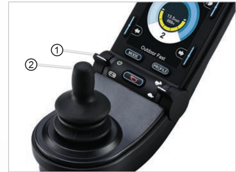
Fig. 66: Blocking the controls
