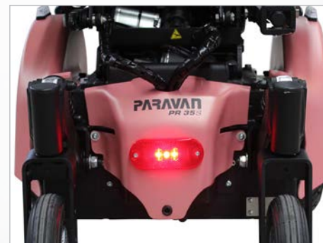
Fig. 10: Illumination at the rear
