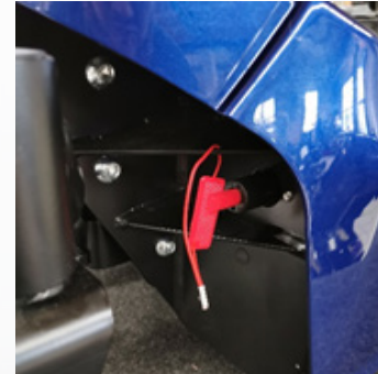
Fig. 98: Battery dicon. switch, inactive
