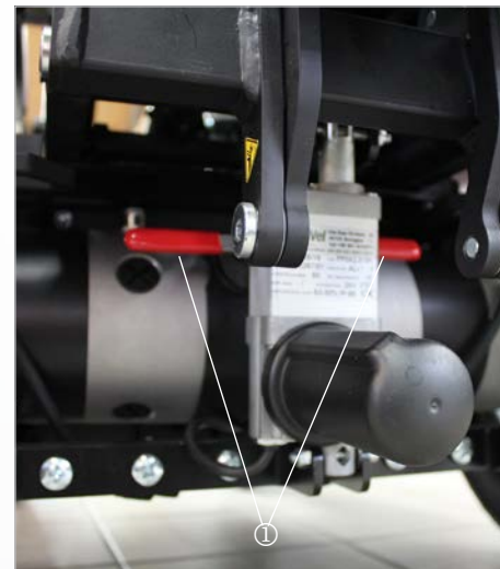
Fig. 25: Brake lock release lever (emergency release)
